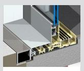
The door sill can be completely recessed into the floor as shown above. For the ultimate finish you can fit a recessed lineal drain on the outside and a retractable roller screen on the inside.
